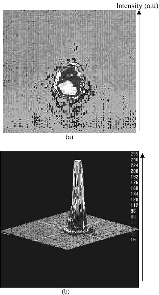
Fig. 4. SPIRICON LBA 300-2D images (a) and 3D images (b) from the SDG1 plate sample, excited by a diode laser at 625 nm.
