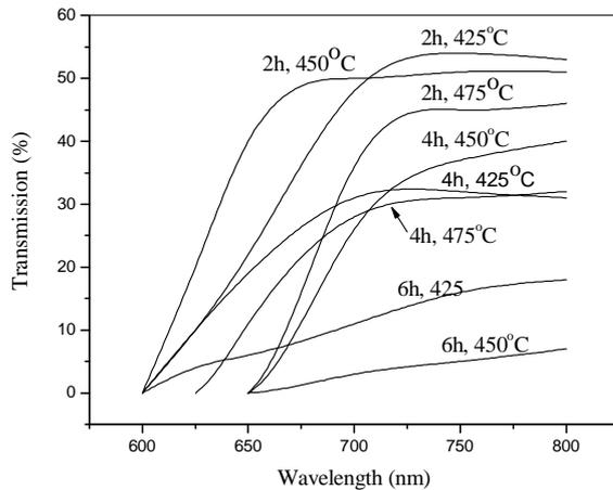
Fig. 2. Transmission spectra of the semiconductor doped glasses belonging to the system  $\text{Li}_2\text{O-Na}_2\text{O-P}_2\text{O}_5\text{-Al}_2\text{O}_3\text{-BaO-SiO}_2\text{-La}_2\text{O}_3$ , doped with 1 wt.%  $\text{CdS}_{0.5}\text{Se}_{0.5}$  and 1 wt.% ZnO (SDG2). The glass samples were annealed for 2h, 4h and 6h at 425 °C, 450 °C and 475 °C.
