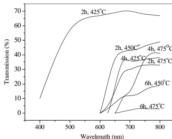
Fig. 1. Transmission spectra of the semiconductor doped glasses belonging to the oxide system Li<sub>2</sub>O-P<sub>2</sub>O<sub>5</sub>-Al<sub>2</sub>O<sub>3</sub>-BaO-SiO<sub>2</sub>-La<sub>2</sub>O<sub>3</sub>, doped with 1 wt.% CdS<sub>0.5</sub>Se<sub>0.5</sub> and 1 wt.% ZnO (SDG1). The glass samples were annealed for 2h, 4h and 6h at 425 °C, 450 °C and 475 °C.
