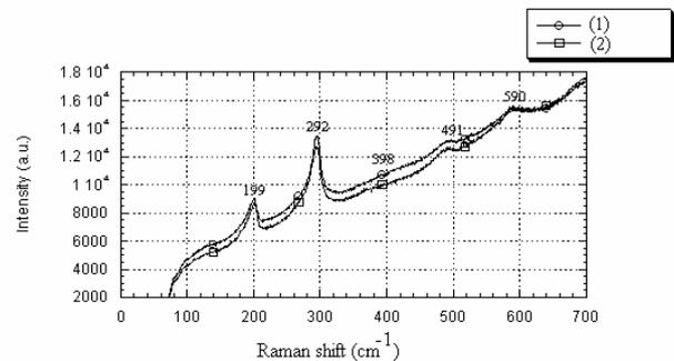
Fig. 3. Raman spectra for SDG1, 2 h annealed (1) and SDG2, 6 h annealed (2), excited at 514.5 nm. The annealing temperature was 450 °C.
