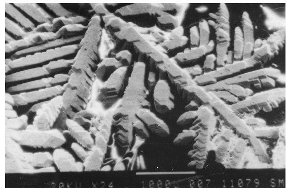
Fig. 6. Mo microdendrites growth on nickel electrode surface at 1023 K.
