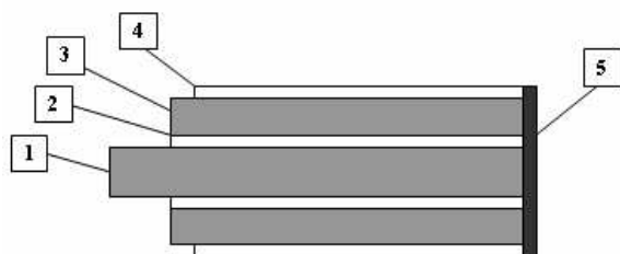
Fig. 3. Sketch of coaxial microthermocouple. 1 - n-type bismuth telluride thermoelectric material in cylindrical glass isolation 2, 3 - other cylindrical coaxial microwire of bismuth telluride of p-type, covered with cylindrical glass isolation 4, connected by hot contact of nickel 5 with hot terminals 1 and 3.
