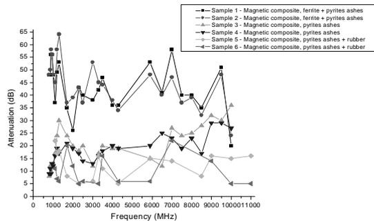
Fig. 2. The attenuation vs. frequencies, for magnetic shields obtained from 50 % ferrite + 50 % pyrites ashes, 100 % pyrites ashes, and pyrites ashes + rubber.
