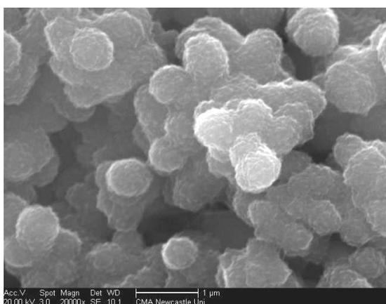
Fig. 7. SEM on a electrodeposited PANI sample by Galvanostatic Method x 20000.
