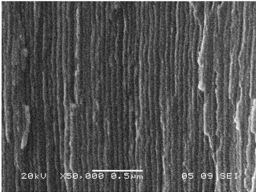
Fig. 1. SEM micrograph of LCMO nanowires obtained using  $\text{Al}_2\text{O}_3$  template.
