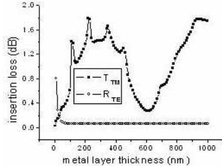
Fig. 2. Insertion loss of TM and TE polarized light ( $T_{TM}$  &  $R_{TE}$ ) as a function of metal layer thickness  $h$ .
