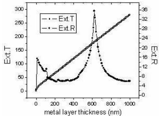
Fig. 3. Extinction ratio of transmission and reflection (Ext.T & Ext.R) as a function of metal layer thickness  $h$ .
