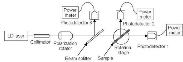
Fig. 7. Schematic diagram of the experimental setup for the efficiency measurement of the fabricated embedded nanograting.
