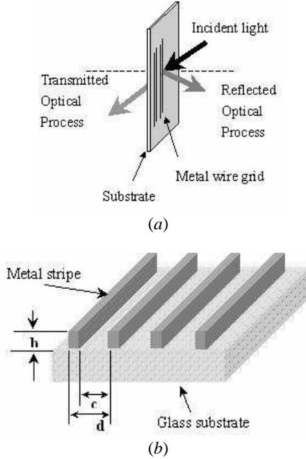
Fig. 1. (a) Schematic of the nanograting PBS, where TM polarized light is transmitted and TE polarized light is reflected. (b) Metal wire nanograting model.
