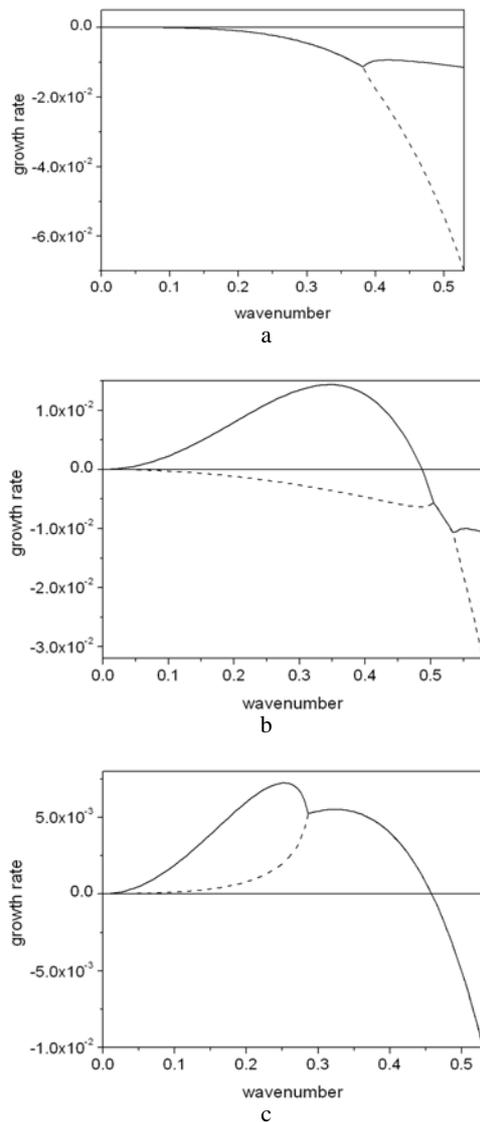
Fig. 2. Growth rate versus wave number computed in the linear approximation with different parameters values for three cases: (a) conductive state; (b) monotonic instability; (c) oscillatory instability.
