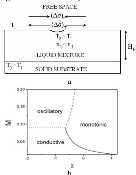
Fig. 1. (a) System sketch: on a solid substrate lies a binary mixture thin liquid film with free upper surface. A temperature gradient  $T_0 > T_1$  is maintained between the lower and upper surfaces; (b) stability diagram for the considered system computed from the linear problem.
