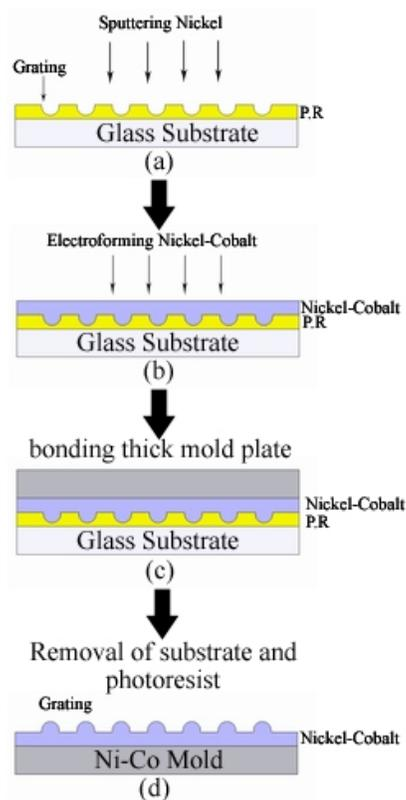
Fig. 2. Electroplating process for Ni-Co grating mold.
