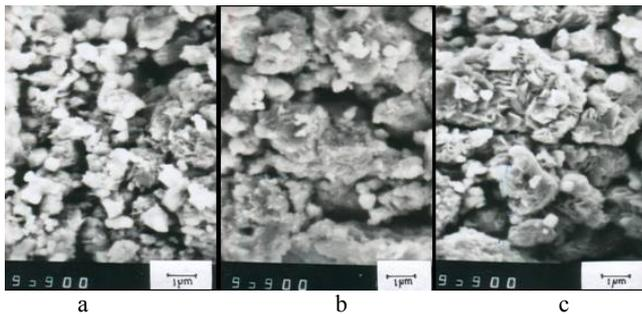
Fig. 3. SEM micrograph of  $\text{SrLa}_{0.2}\text{Fe}_{11.8}\text{O}_{19}$  annealed at 900 °C for different annealing time: a) 10 minutes; b) 40 minutes; c) 320 minutes.
