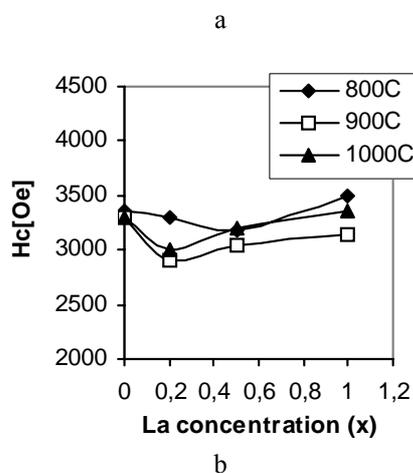
Fig. 1. The effect of La concentration and annealing temperature on magnetic properties of SrLa<sub>x</sub>Fe<sub>12-x</sub>O<sub>19</sub> hexaferrites ( $0 \leq x \leq 1$ ) (annealing time is 40 minutes).
