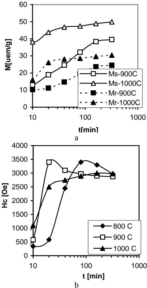
Fig. 2. The effect of annealing time on the magnetic parameters: magnetization (a) and coercivity (b) of  $SrLa_{0.02}Fe_{11.8}O_{19}$  annealed at 800, 900 and 1000 °C.
