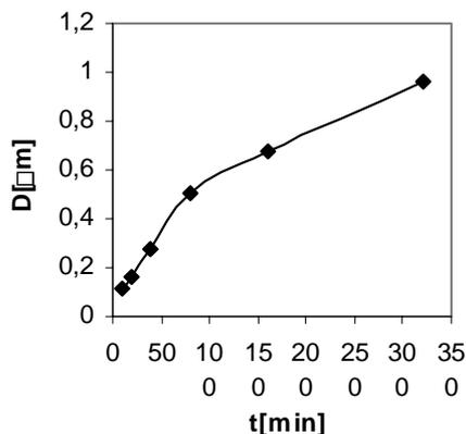
Fig. 5. The dependence of grain size  $D$  on annealing time  $t$  for  $\text{SrLa}_{0.2}\text{Fe}_{11.8}\text{O}_{19}$  annealed at 900 °C.
