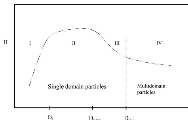
Fig. 7. Qualitative dependence of  $H_c$  on the average grain size  $D$ . The four zones are determined by the three diameters: for the thermal activation ( $D_i$ ), transition to inhomogeneous rotation ( $D_{\text{trans}}$ ) and the formation of multidomain particles ( $D_{\text{crit}}$ ).
