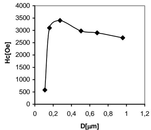
Fig. 6. The dependence of coercivity  $H_c$  on grain size  $D$  for  $\text{SrLa}_{0.2}\text{Fe}_{11.8}\text{O}_{19}$  annealed at 900 °C.
