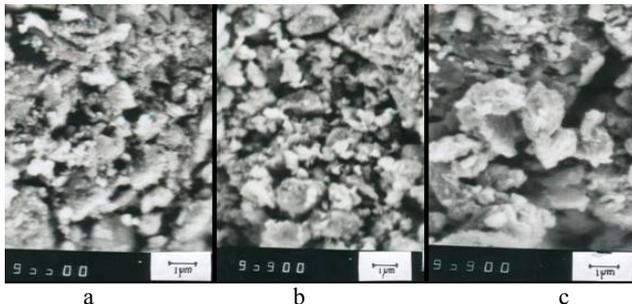
Fig. 4. SEM micrograph of  $\text{SrFe}_{12}\text{O}_{19}$  for different annealing temperature: a) 800 °C; b) 900 °C; c) 1000 °C; annealing time is 40 minutes.
