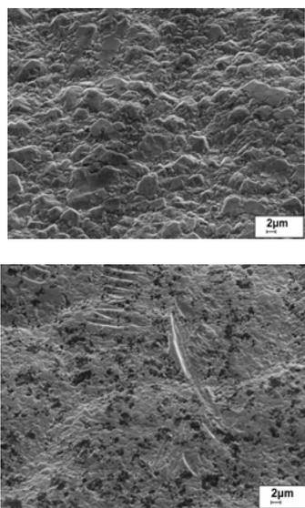
Fig. 6. SEM images of nickel electrodeposition for 5 g/l (top) and 10 g/l (bottom) alumina concentration.
