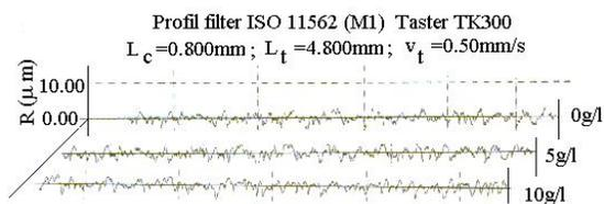
Fig. 4. Influence of the alumina concentration on micro geometry of electrodeposited film.
