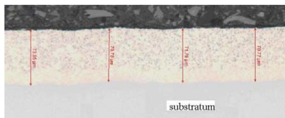
Fig. 3. General view of electrodeposited film of nickel / alumina nanoparticles.
