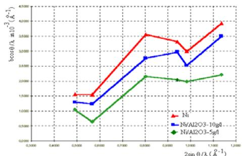
Fig. 9. Dependence of the mosaic block dimension versus the interplanar distance.
