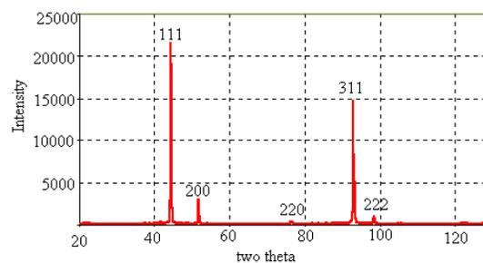
Fig. 8. X-ray diffraction spectrum of electrodeposited nickel film with 10% alumina nanoparticles.
