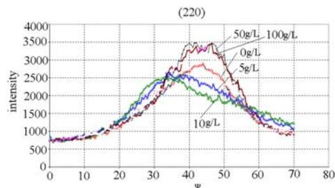
Fig. 11. Dependence of the X-ray diffraction intensity versus the incidence angle of X-ray beam
