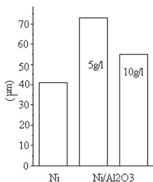
Fig. 5. Thickness of Ni/Al<sub>2</sub>O<sub>3</sub> composite coatings
