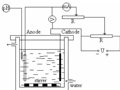
Fig. 1. Electroplating cell and electrode arrangement.
