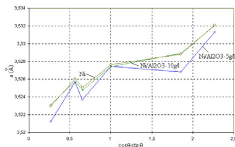
Fig. 10. Extrapolation curves for determining the lattice parameter,  $a$ , for nickel electrodeposited.
