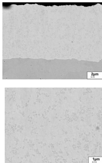
Fig. 2. Cross views of the electrodeposited film of nickel / alumina nanoparticles
