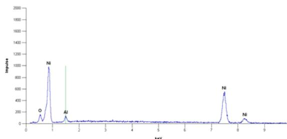
Fig. 7. EDXS spectrum of electrodeposited film.
