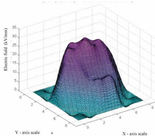
Fig. 2. Surface plot of the reconstructed electric field for a non-symmetrical electrode system.
