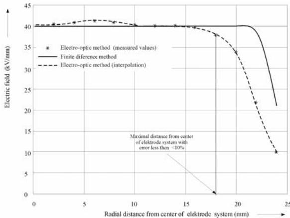
Fig. 1. Electric field strength vs. distance from the center of electrode system (numerical approach using FDM (finite difference method), normal experimental approach (direct tomographic reconstruction), enhanced experimental approach (tomographic reconstruction with zooming)).
