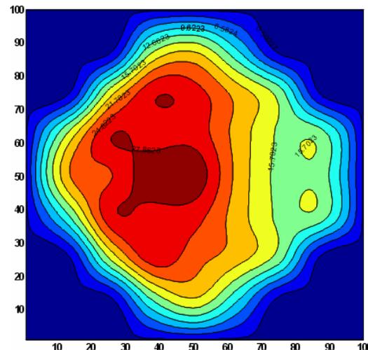
Fig. 3. Contour plot of the reconstructed electric field for a non-symmetrical electrode system.
