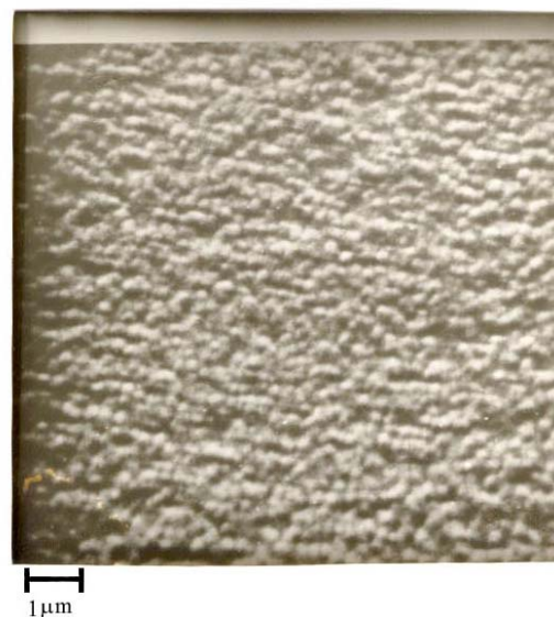
Fig. 3. Scanning electron microscope image of CdS film, ( t = 100 \text{ nm} , T_s = 200^\circ\text{C} , R = 15 \text{ nm/s} ).
