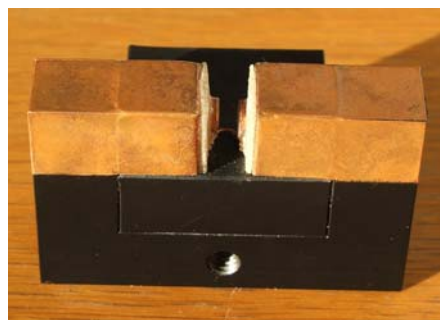
Fig. 3. The NMR-MOUSE used for in situ measurements at a stress-strain device.
