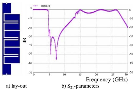
Fig. 3. An example of low-pass filter with the same cell shape as published in [6].
