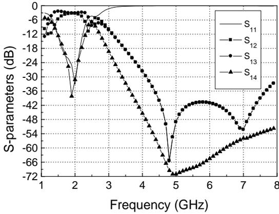
Fig. 6. Simulated results of the proposed rat-race hybrid ring in wide frequency range.
