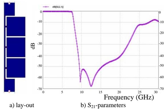
Fig. 4. An example of low-pass filter with the proposed cell shape.
