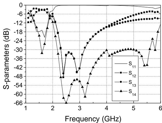
Fig. 2. Simulated results of the rat-race hybrid ring published in [6] in wider frequency range. Substrate thickness  $h = 0.508$  mm, relative dielectric constant  $\epsilon_r = 2.1$  and outer radius 11.2 mm.
