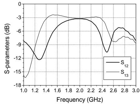
b) Measured  $S_{12}$  and  $S_{13}$  parameters
