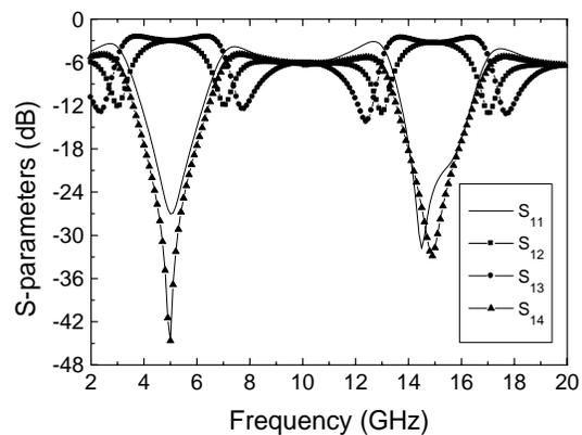
Fig. 1b. S-parameters of the conventional rat-race hybrid ring with the outer radius 11.2 mm.
