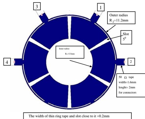
Fig. 5. Lay-out of the proposed rat-race hybrid ring (angles between neighbouring ports are  $60^\circ$ ).
