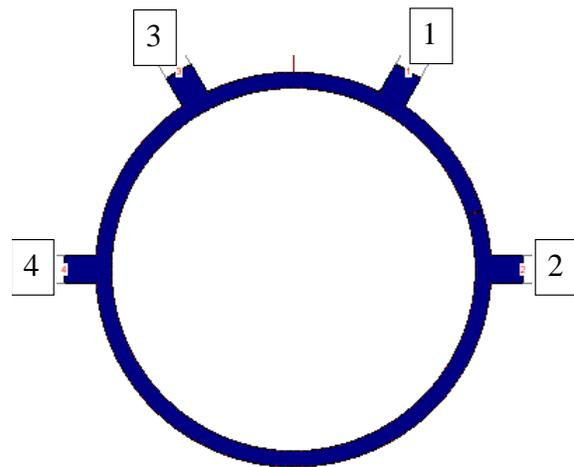
Fig. 1a. Lay-out of the conventional rat-race hybrid ring.
