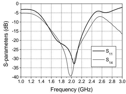
a) Measured  $S_{11}$  and  $S_{14}$  parameters
