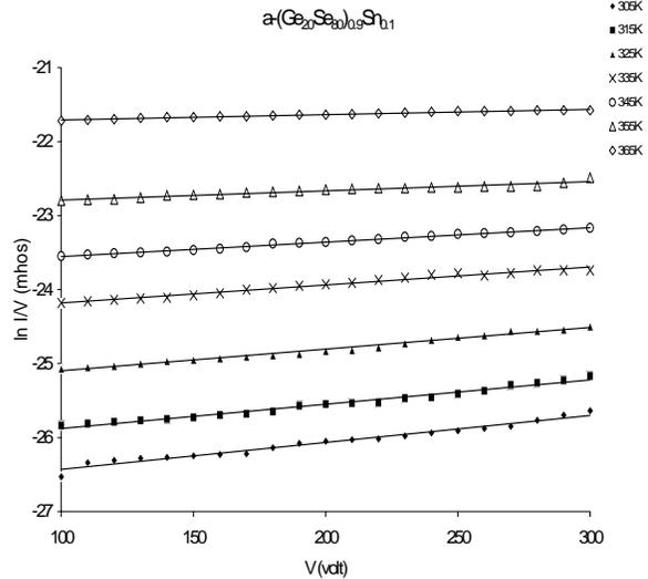
Fig. 1. Plots of  $\ln I/V$  vs. V curve for a-  $(\text{Ge}_{20}\text{Se}_{80})_{0.90}\text{Sn}_{0.10}$  at different temperatures.
