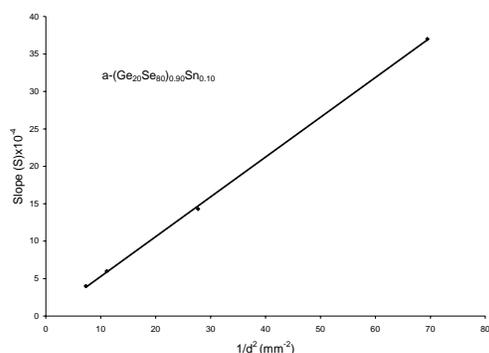
Fig. 4.  $S$  vs.  $1/d^2$  curve for different electrode gaps for  $(\text{Ge}_{20}\text{Se}_{80})_{0.90}\text{Sn}_{0.10}$  glassy system.
