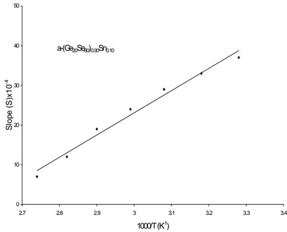
Fig. 2. Plots of  $S$  vs.  $1000/T$  curve for  $(\text{Ge}_{20}\text{Se}_{80})_{0.90}\text{Sn}_{0.10}$  glassy system.
