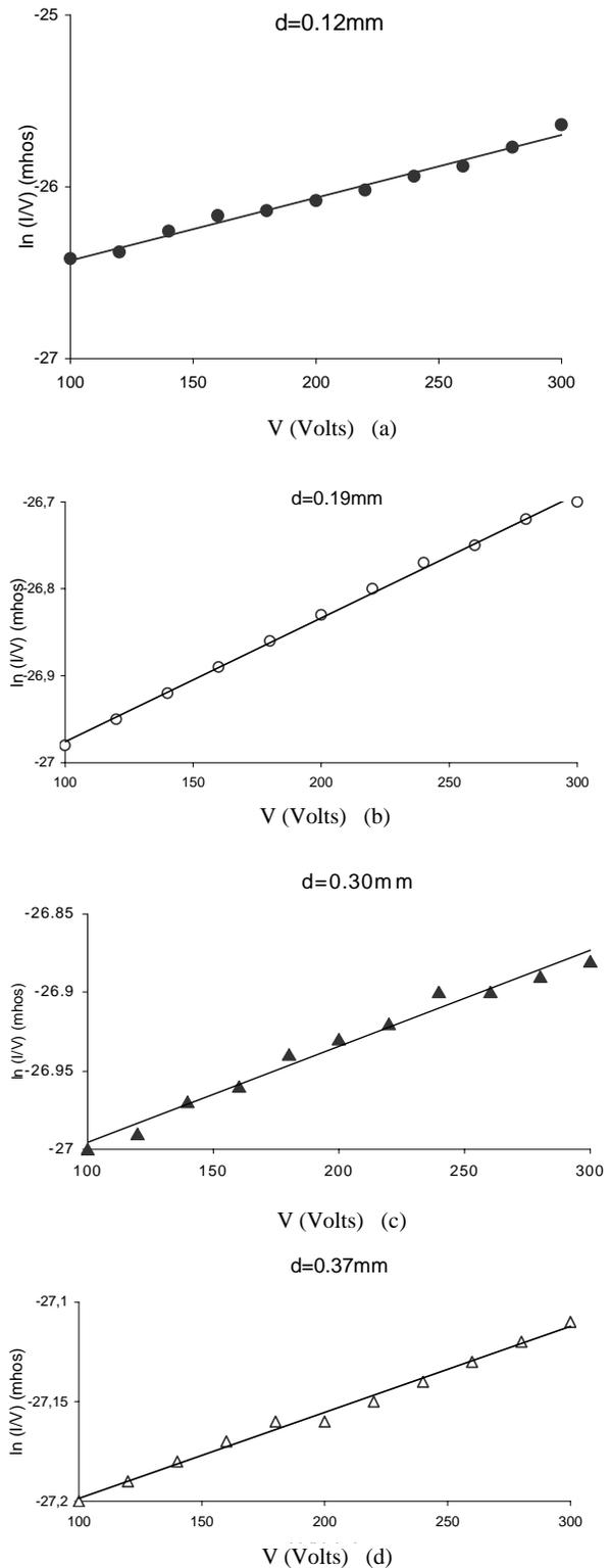
Fig. 3. Plots of  $\ln I/V$  vs.  $V$  curve at room temperature having different electrode gaps for  $(\text{Ge}_{20}\text{Se}_{80})_{0.90}\text{Sn}_{0.10}$  glassy system.
