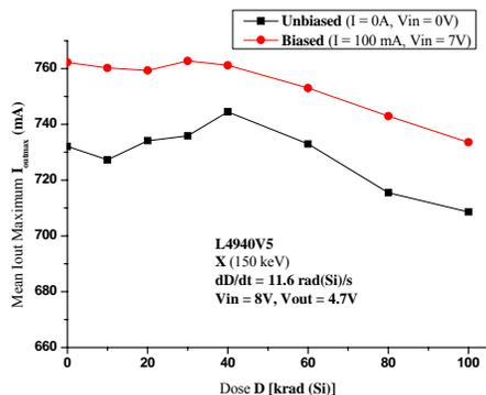
Fig. 2. Change of maximum output current on serial transistor of voltage regulator L4940V5 under influence of X radiation.
