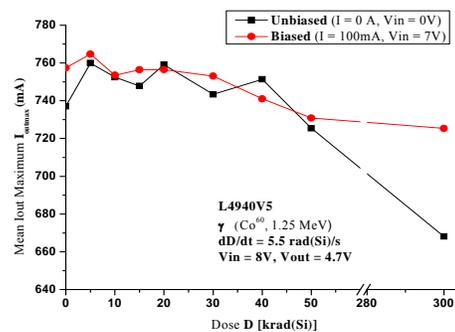
Fig. 1. Change of maximum output current on serial transistor of voltage regulator L4940V5 under influence of  $\gamma$  radiation.
