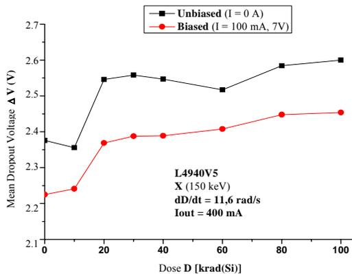
Fig. 6. Change of mean dropout voltage on serial transistor of voltage regulator L4940V5 under influence of X radiation.
