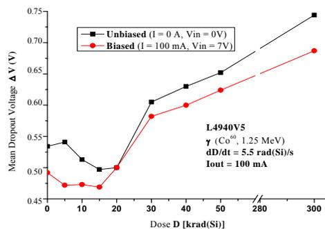
Fig. 3. Change of mean dropout voltage on serial transistor of voltage regulator L4940V5 under influence of  $\gamma$  radiation.
