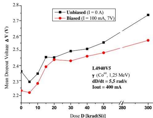
Fig. 5. Change of mean dropout voltage on serial transistor of voltage regulator L4940V5 under influence of  $\gamma$  radiation.
