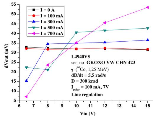
Fig. 8. Line regulation characteristics of biased voltage regulator L4940V5 after exposure to  $\gamma$  radiation dose of 300 krad(Si).
