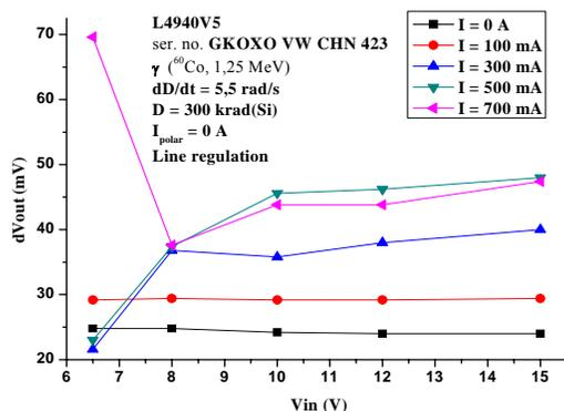
Fig. 7. Line regulation characteristics of unbiased voltage regulator L4940V5 after exposure to  $\gamma$  radiation dose of 300 krad(Si).
