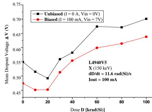
Fig. 4. Change of mean dropout voltage on serial transistor of voltage regulator L4940V5 under influence of X  $\gamma$  radiation.
