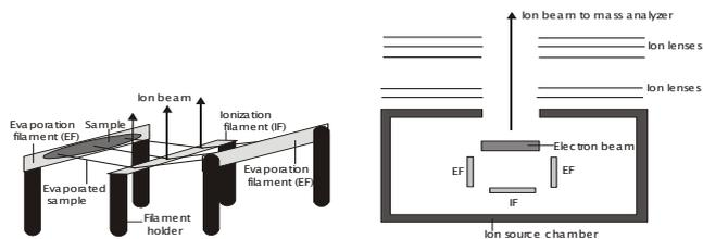
Fig. 1. Schematic diagram of a triple filament surface ionization source with electron impact source. Electron beam is perpendicular to the paper.
