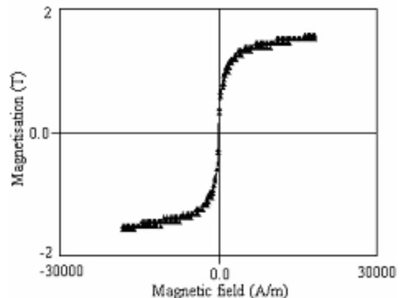
Fig. 3. Axial hysteresis loop for the as-cast  $Fe_{77.5}Si_{7.5}B_{15}$  amorphous ribbons.
