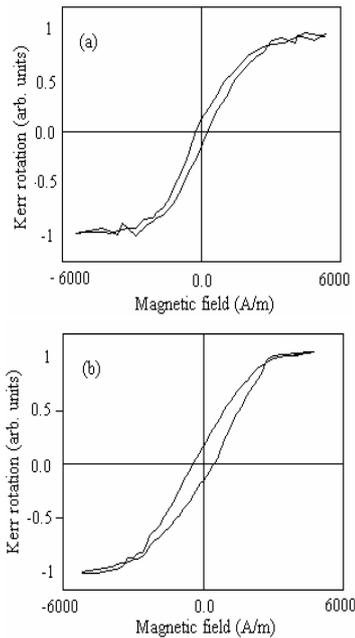
Fig. 1. Longitudinal Kerr hysteresis loops for the as-cast  $Fe_{77.5}Si_{7.5}B_{15}$  amorphous ribbons with the external field parallel to the ribbon longitudinal axis: (a) free side; (b) wheel side.
