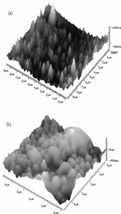
Fig. 2 (a and b). Presents the typical atomic force images for the free and wheel side, respectively. It is well known that the magneto-optical response of a material is strongly dependent on its microstructure and morphology. The surface topography images presented in Fig. 2 show two different kind of topographies for the free and wheel side.
