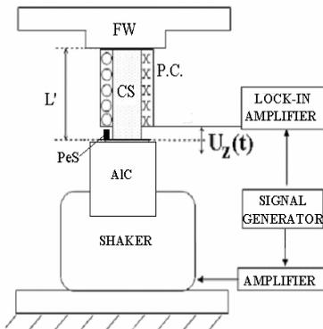
Fig. 2. Experimental arrangement used to study the elastomagnetic response of the composite sample under external dynamic deformation produced by a shaker. FW = fixed wall, P.C. = pick-up coil, CS = composite sample, AIC = aluminium cylinder, PeS = piezoelectric sensor,  $L'$  = pre-stressed sample length,  $L-L' > D$ ,  $U_2(t) = D \sin(2\pi\nu t)$  = dynamic longitudinal deformation induced by the shaker vibration.
