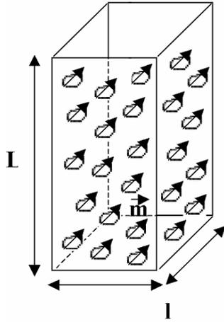
Fig. 1. Schematic view of the elastomagnetic composite sample (length,  $L=4.5 \times 10^{-2}$  m and width,  $l=5 \times 10^{-3}$  m).  $m$  – permanent magnetic moment of the  $\text{Sm}_2\text{Co}_7$  micro - particles.
