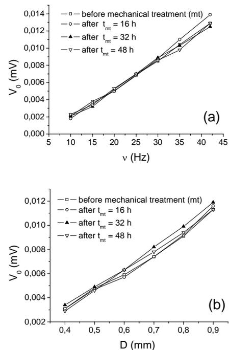
Fig. 5. Elastomagnetic response of the sample,  $V_o$ , as function of frequency,  $\nu$  (at fixed  $D=0.7$  mm) (a) and amplitude,  $D$  (at fixed  $\nu=30$  Hz) (b), of the dynamic mechanical solicitation.  $V_o$  vs.  $\nu$  and  $D$  were registered after 16, 32 and 48 h of dynamic mechanical treatment at  $\nu=30$  Hz and  $D=0.7$  mm.
